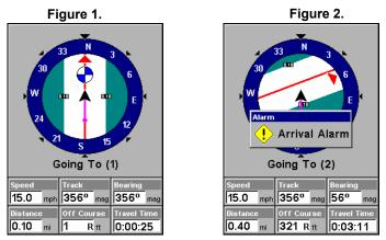
Navigating along a route: Fig. 1 shows the Navigation Page at the start of a route, heading straight for the first waypoint (Wpt 1). In Fig. 2, the traveler has arrived at Wpt 1; the arrival alarm has been triggered and the bearing arrow on the compass rose has turned to point toward Wpt 2, off to the northeast.
